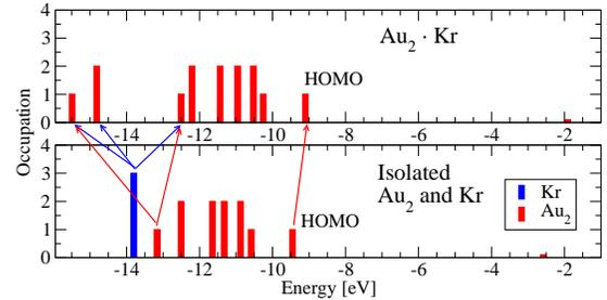
**Figure 3.** Evolution of self-consistent  $GW$  spectra from isolated  $\text{Au}_2$  and Kr to relaxed  $\text{Au}_2\text{Kr}$ .
