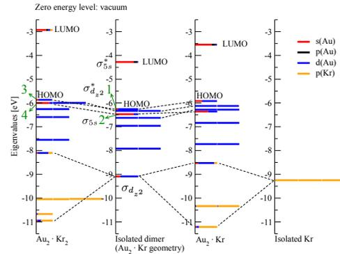
**Figure 2.** Molecular-orbital picture based on atom- and angular-momentum-projected (PBE) electronic density of states, calculated for Kr bonding to  $\text{Au}_2$ . The dashed lines link similar orbitals in different molecular arrangements. The labels 1 to 4 denote orbitals used to calculate the change in the partial electron density upon addition of two Kr to  $\text{Au}_2$ , shown in Fig. 4.
