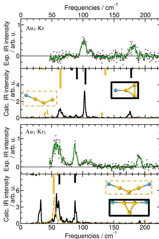
**Figure 1.** FIR-MPD<sup>9</sup> (upper panels) and theoretical IR spectra<sup>9</sup> (lower panels) at  $T = 100$  K. Theoretical harmonic spectra are also shown (as upside-down bars in the lower panels) for the two isomers of  $Au_3Kr$  (top) and  $Au_3Kr_2$  (bottom). The yellow (dashed) lines refer to the obtuse-angled isomer, while the black lines refer to the acute-angled one.
