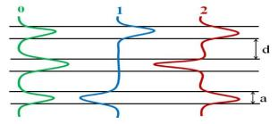
FIG. 1: (Color online) Schematic diagram of an array of three identical single mode waveguides and the field distributions of the three normal modes.
