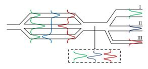
FIG. 3: (Color online) Schematic of waveguide structure describing the how the modes are separated at output.
