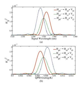
FIG. 6: (Color online) Variation of the efficiency of the three down conversion processes (a) as a function of signal wavelength; (b) as a function of QPM grating.
