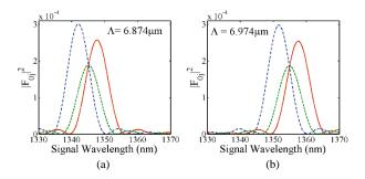
FIG. 7: (Color online) Variation of the efficiency of the three down conversion processes as a function of signal wavelength having grating period (a)  $\Lambda = 6.874 \ \mu\text{m}$ ; (b)  $\Lambda = 6.974 \ \mu\text{m}$
