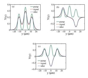
FIG. 4: (Color online) Normalized transverse modal field distributions along y - direction in a three waveguide coupler (a) fundamental symmetric normal mode (0) at pump, signal and idler wavelengths; (b) fundamental symmetric mode normal mode (0) at pump wavelength and the first excited anti symmetric normal mode (1) at signal and idler wavelengths; (c) fundamental symmetric mode normal mode (0) at pump wavelength and the second excited symmetric normal mode (2) at signal and idler wavelengths
