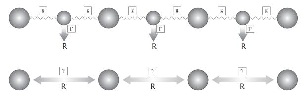
**Figure 1.** (above) A scheme of bipartite tight-binding spin-chain with some elements subjected to strong loss. This scheme is described by Eq. (11). (below) A scheme of dissipatively coupled tight-binding spin chain described by Eq. (1).
