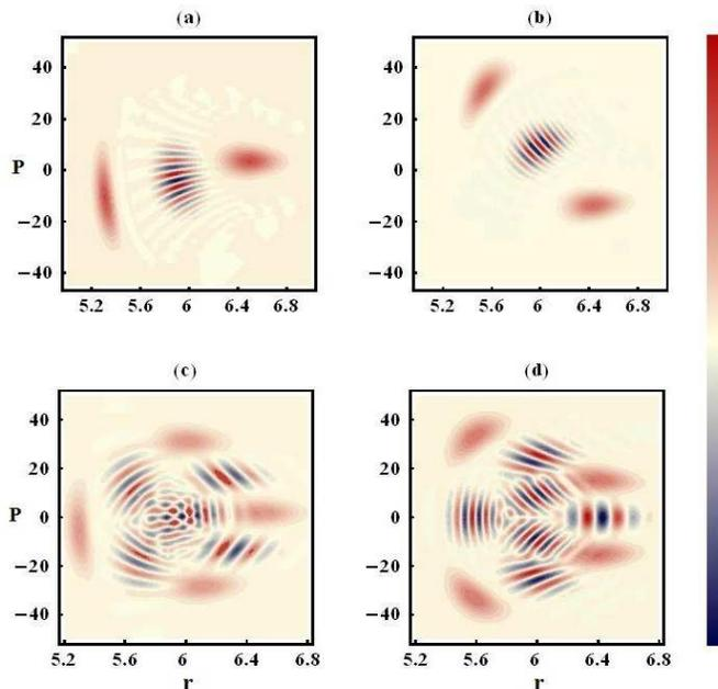
FIG. 6: (Color online) Time evolution of Wigner function of the CS. The first row shows cat-like state at  $t = T_{\text{rev}}/4$  for (a)  $j = 0$ , and (b)  $j = 82$  and the second row shows compass-like state at time  $t = T_{\text{rev}}/8$  for (c)  $j = 0$ , and (d)  $j = 64$ . The mesoscopic superposition of maximum sensitivity in Rotating Morse potential
