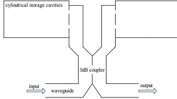
Fig.1. Schematic of the SLED type pulse compressor
