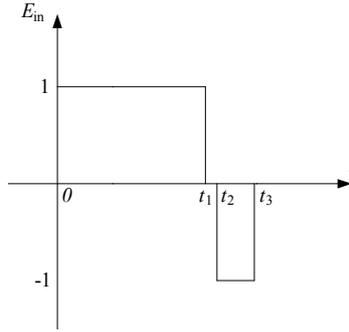
Fig. 6. Schematic of the normalized input field with PSK which have no power output during the phase shifting process
