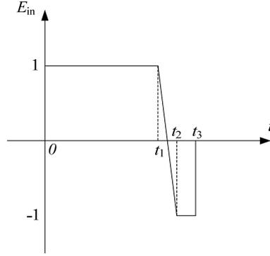
Fig.4. Schematic of the normalized input field with slow PSK
