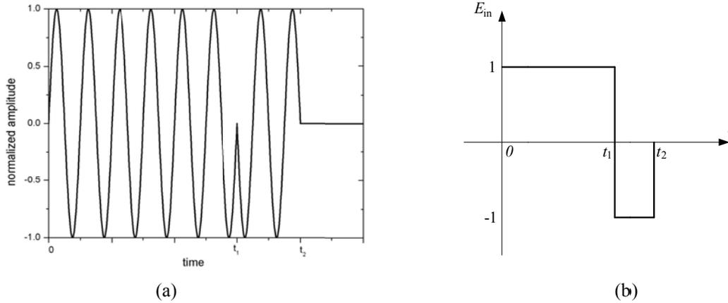
Fig.2. Schematic of the input field with ideal PSK
