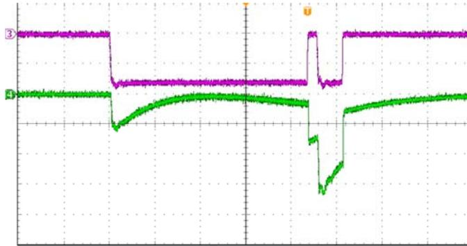
Fig.8. Test waveform of SLED with nonideal PSK
