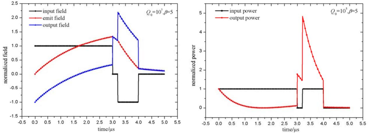
Fig. 7. Normalized field and power of SLED using PSK without power output during the phase shifting process
