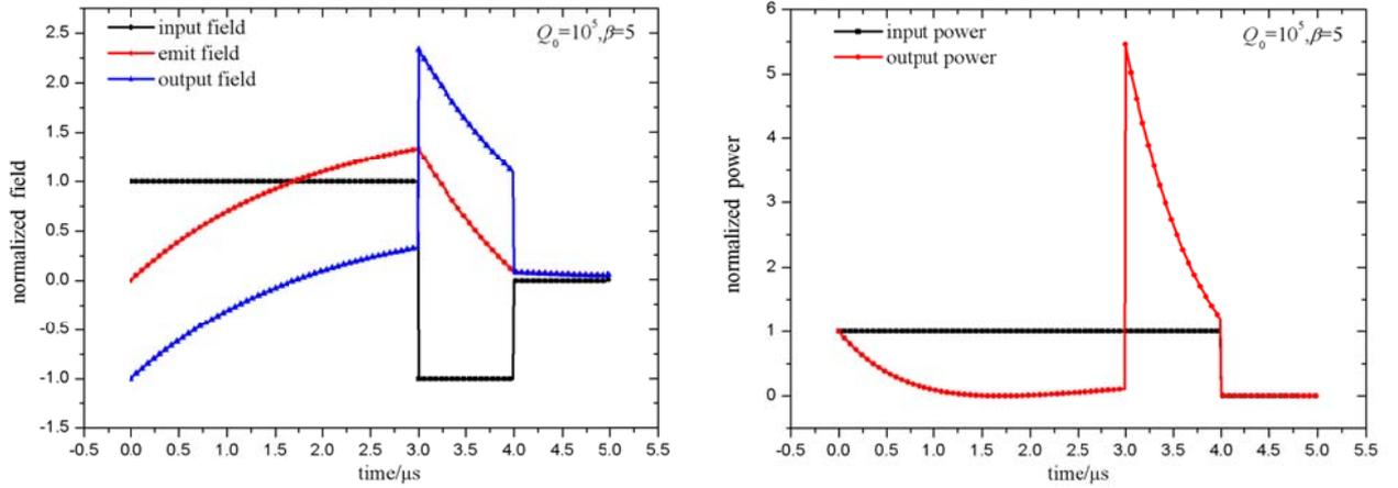
Fig.3. Normalized field and power of SLED with ideal PSK
