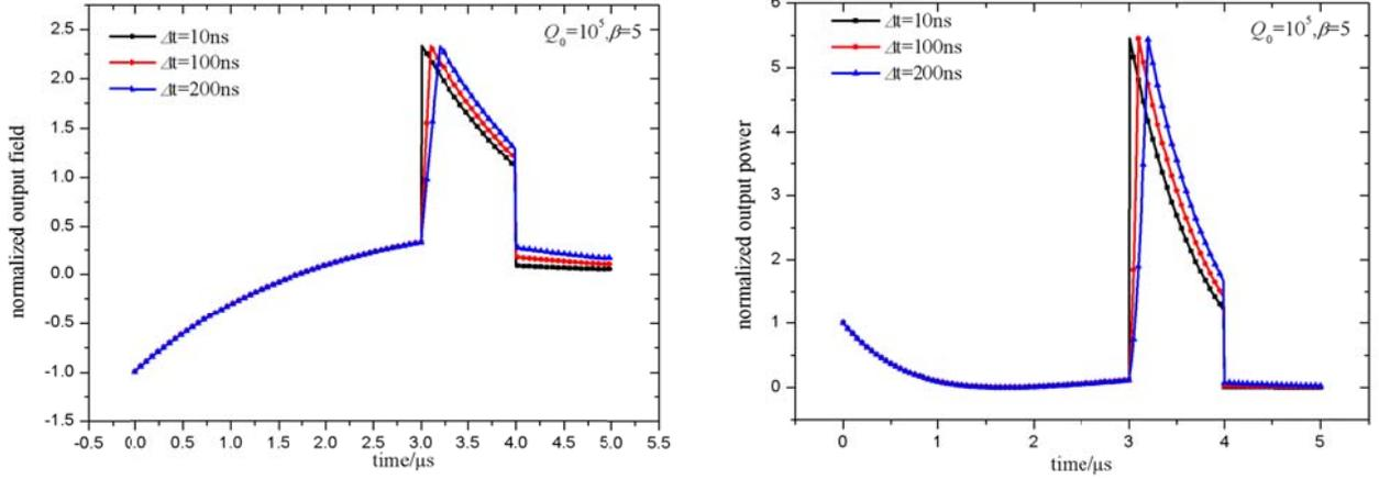
Fig.5. Normalized output field and power of SLED using PSK with different switching speed
