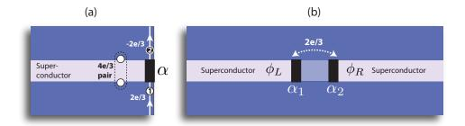
FIG. 3. Detection schemes for parafermion zero modes, illustrated using the  $\nu=2/3$  setup from Fig. 2(a). (a) Hybridizing a zero mode with the gapless edge states generates 'perfect Andreev conversion'. (b) Coupling  $\mathbb{Z}_3$  parafermions across a Josephson junction yields a current (mediated by 2e/3 tunneling)  $6\pi$ -periodic in the phase difference  $\phi_L - \phi_R$ .
