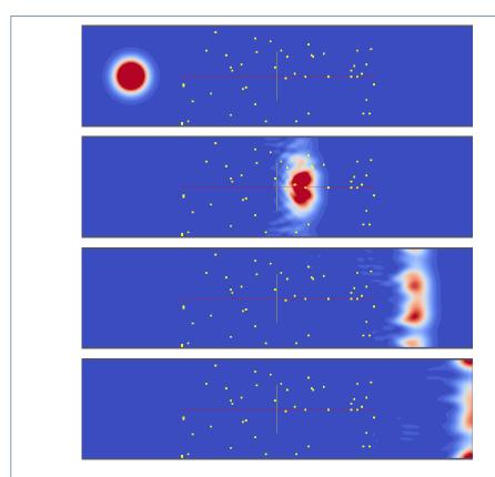
Figure 2 Wave packet density  $\rho$  at times  $=0,\,900,\,1500,\,$  and 1800 (lattice units) for a Gaussian wave packet propagating through a graphene sample with randomly distributed impurities. The simulation is performed with impurity percentage C=0.5% and impurity potential V=50 MeV.
