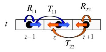
Figure 1 Sketch of the transfer and residency matrix elements.  $T_{11}$  is the fraction of up-moving spinor jumping from j-1 at time n-1 to j at time n, while  $R_{11}$  is the fraction left in j-1.  $T_{22}$  and  $R_{22}$  bear the same meaning for the down moving spinor.
