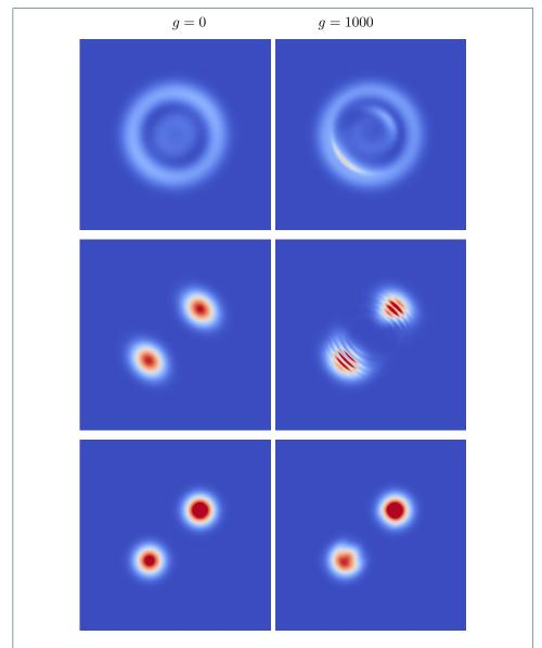
Figure 3 Wave packet density  $\rho=|\psi_1|^2+|\psi_2|^2+|\psi_3|^2+|\psi_4|^2$  for the scheme solving Dirac equation with NJL interaction. These snapshots are taken at time t=200 for  $k=0.004,\,0.04$  and 0.4 (from top to bottom). The figure shows how the initial energy affects the separation phenomenon. In particular, at low energy, k=0.004, no splitting of the wavepackest is observed.
