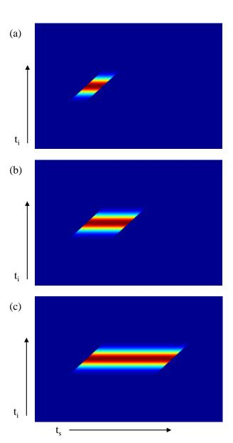
FIG. 2. Joint temporal amplitudes when the idler and pump are group velocity matched. For increasing fibre length compared to the length of the pump pulse  $\tau$ , the group velocity walk-off of the signal smears out the JTA. (a)  $\beta_{1s}L/\tau=2$  (b)  $\beta_{1s}L/\tau=5$  (c)  $\beta_{1s}L/\tau=10$ .
