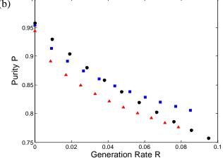
FIG. 9. Purity against generation rate R for different strengths of dispersion, with an initial pump bandwidth of 1nm. R=0 corresponds to the case with no non-linear phase modulation. (a) L=0.5m,(b) L=1m. In each case, black circles: no dispersion; blue squares: realistic dispersion; red triangles: double strength dispersion. Surprisingly, at higher rates the dispersive case sometimes does better than the case with no dispersion.
