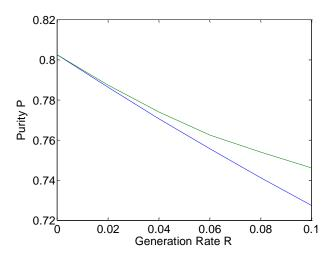
FIG. 6. Purity against generation rate for the symmetric scheme. Blue:  $\tau$  is kept constant. Green:  $\tau$  is increased with R to reoptimise. Again, the phase modulation reduces P as R is increased, though here P is lower to start with than in the asymmetric scheme because there is more correlation in the sinc ripples of the JSA.
