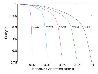
FIG. 7. Purity as a function of the effective generation rate, RT, when filtering is applied to one of the photons (the herald) resulting in transmission T. Unfiltered generation rates R are shown from 0.02 to 0.1.
