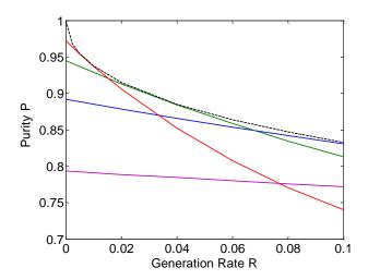
FIG. 4. Purity plotted against generation rate for four choices of fibre parameters. Red:  $\beta_{1s}L/\tau=40$ . Green:  $\beta_{1s}L/\tau=20$ . Blue:  $\beta_{1s}L/\tau=10$ . Purple:  $\beta_{1s}L/\tau=5$ . The black dashed line shows the purity varying with generation rate after numerical optimization of  $\beta_{1s}L/\tau$ . It can be seen a large value of  $\beta_{1s}L/\tau$  is desirable at low rates, but for higher rates it will cause a more rapid fall-off in purity.
