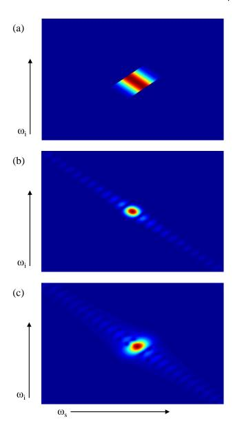
FIG. 5. (a) Joint temporal amplitude when the signal and idler are equally spaced in  $\beta_1$  about the pump. The pump duration is optimised to avoid correlation, but the hard edges to the JTA caused by the sudden beginning and end of the nonlinearity mean that some correlation is inevitable. (b) Corresponding JSA with low generation rate. (c) At higher generation rate, R=0.2, showing the effects of SPM and XPM. The JSA is broadened in one direction.
