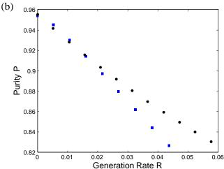
FIG. 10. Purity against generation rate with anomalous dispersion, for an initial pump bandwidth of 2nm. (a) L=0.5m,(b) L=1m. In each case, black circles: no dispersion; blue squares: realistic dispersion. Here, a very slight benefit can be seen at low rate for the dispersive case compared to the case without dispersion.
