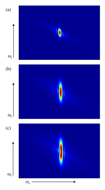
FIG. 3. JSA for different generation rates R, showing the effect of SPM and XPM. The initial effect is to broaden the idler, eventually leading to a splitting and distortion of the JSA which reduces the purity P. (a) R approaching zero, P=89% (b) R=0.1, P=83% (c) R=0.2, P=78%.
