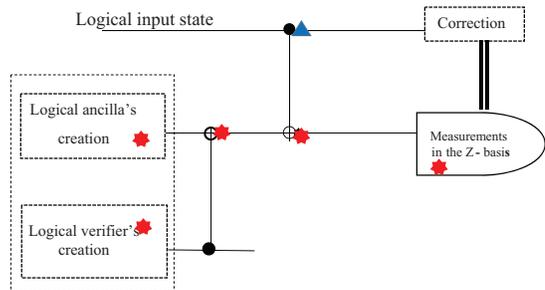
FIG. 1. A schematic diagram for a “noisy” QEC for correction of  $X$  errors, where the star represents the location where a syndrome error might occur, and the triangle a location where a correction error might occur. The Steane ancilla state must be prepared in the  $|+L\rangle$  and the measurements performed in the Z-basis.
