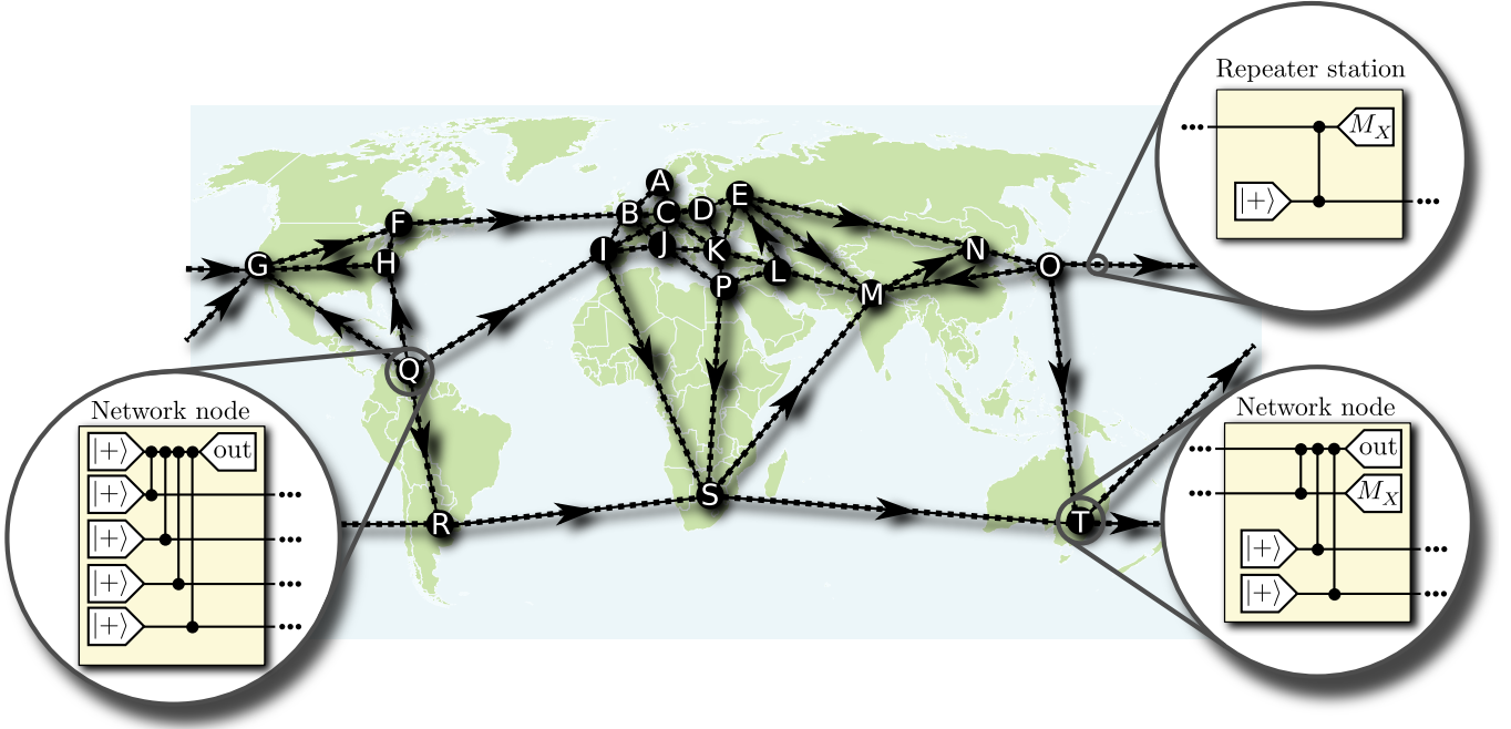
FIG. 1. Multipartite quantum network based on graphs: network nodes together with links between them constitute a graph. Both network nodes and repeater stations receive and send quantum particles. They prepare qubits (in the |+\rangle -state), perform entangling quantum gates ( C_Z -gates) and measurements (in the X -basis). The number of such actions for a given node depends on its number of neighbours. Arrows indicate the transmission direction. Some examples are illustrated. Note that repeater stations have exactly two neighbours, while network nodes may have more than two neighbours.
