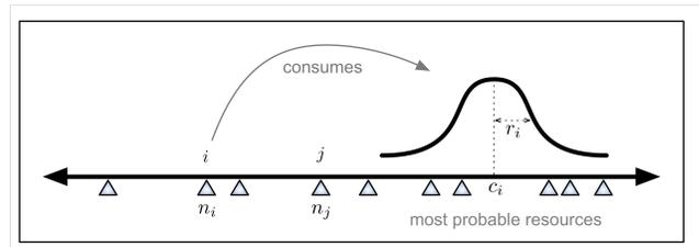
**FIG. 3. Schematic of the probabilistic niche model (PNM).** Each species  $i$  has some position  $n_i$  in a latent niche space, represented here by a one-dimensional axis. Species  $i$  consumes each other species  $j$  (located at  $n_j$ ) with a probability given by a Gaussian function centered at a preferred feeding location  $c_i$  and width  $r_i$ . Taxa whose niche positions are nearer the preferred feeding location are consumed with higher probability.
