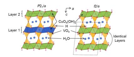
FIG. S1: Crystal Structures of the  $P2_1/a$  (left) and I2/a (right) structures of volborthite, which are shown by coordination polyhedra viewed along the *b* axis. The unit cells are shown by the black dotted lines.
