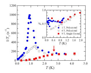
FIG. S3: Temperature dependences of  $1/T_1$  at 1 T (blue dots) and 6 T (black circles) for the polycrystalline sample and at 9 T (red squares) for the single crystal. The data for the polycrystalline sample are taken from Ref. [1]. In the single crystal measurements, the magnetic field was applied perpendicular to the *ab* plane. The arrow indicates the transition temperature of 2.7 K at 9 T for the single crystal. The inset shows the temperature dependences of the stretch exponent  $\beta$ .
