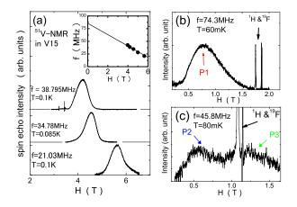
FIG. 3: (Color online) (a)  ${}^{51}$ V-NMR spectra for the V<sup>4+</sup> ions in the triangle observed in its  $S_{\rm T}=3/2$  ground states at very low temperature for three different resonance frequencies. The inset shows the external field dependence of resonance frequency for the peak measured below 100 mK. Typical  ${}^{51}$ V-NMR spectra observed in the  $S_{\rm T}=1/2$  ground states are shown in (b) and (c).
