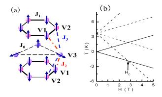
FIG. 2: (Color online) (a) Schematic view of the relative positions of V<sup>4+</sup> (s = 1/2) ions (solid circles) and the exchange coupling scheme in the V15. (b) Magnetic energy level scheme of the V15 as a function of the external magnetic field. Solid and broken lines show the nearly degenerated two  $S_{\rm T} = 1/2$ branches and the  $S_{\rm T} = 3/2$  branches, respectively.
