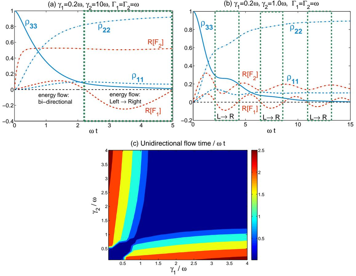
FIG. 2: (Color online) (a) and (b) Population dynamics of the three states in the  $\Lambda$  system, as well as our measure for energy flow,  $\mathcal{R}[F_j(t)]$  with  $\Gamma_1 = \Gamma_2$ ,  $\gamma_1 = 0.2\omega$  and different values for  $\gamma_2$ : (a)  $\gamma_2 = 10\omega$ , (b)  $\gamma_2 = \omega$ . The  $L \rightarrow R$  notation indicates that the unidirectional flow proceeds from the left bath to the right one within the marked frames
