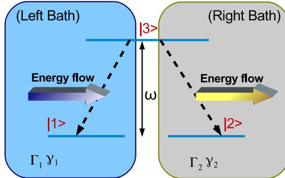
FIG. 1: Schematic representation of our model, a degenerate  $\Lambda$ -type three-level system coupled to two zero-temperature uncorrelated baths characterized by different memory parameters  $\gamma$  and coupling constants  $\Gamma$ .
