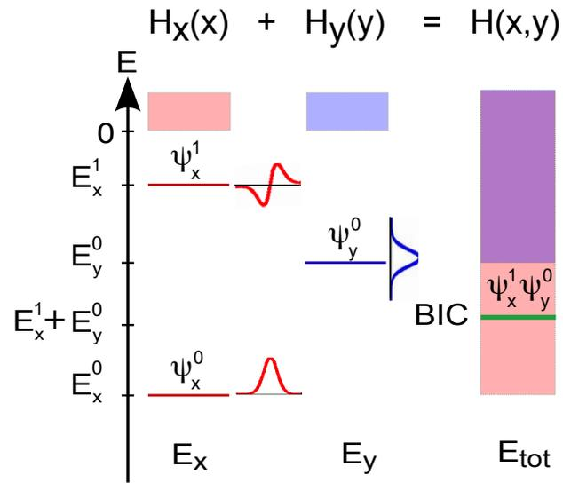
FIG. 1: A schematic illustration demonstrating the concept of a separable BIC in two dimensions.
