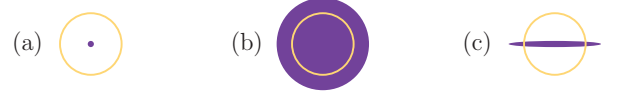
FIG. 2: Pictogram of the three different cases (a)-(c) considered in this letter. The circle (orange) is the cross section of the pump beam at its waist, and the filled circle/ellipse (purple) is the cross section of the probe beam.
