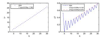
FIG. 3. Dependence between the phase transition value of T (i.e.  $T^*$ ; *left panel*) or the width of the hysteresis (i.e.  $\Delta T$ ; *right panel*) and the number of neighbors (i.e. q).
