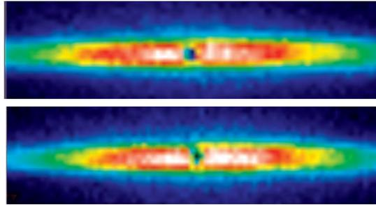
Fig 6: (Color online) The upper panel illustrates absorption of a tightly focused probe beam on the  $F_0 = 2 \rightarrow F = 3$  transition of  $^{87}\text{Rb}$ , as measured in forward scattering. The lower panel shows the influence of a light shift laser on the process; the noticeably smaller dark spot, which shows the modified attenuation of the probe beam, is several microns in diameter.
