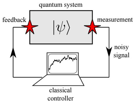
**Fig. 1.** Generic sketch for a closed-loop feedback scheme, in which we wish to control the dynamics of a given quantum system. Note that the feedback loop itself is actuated by a classical controller, i.e., the information after the measurement is *classical* (it is a number and not an operator). Nevertheless, to obtain the correct dynamics of the quantum system one needs to pay additional attention to the measurement and feedback step.
