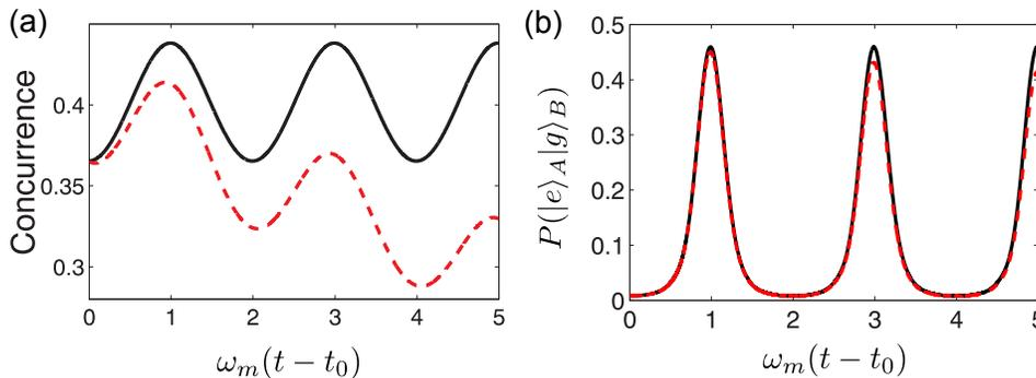
FIG. 3. (a) Time evolution of entanglement of two qubits in terms of concurrence with (dashed line) and without (full line) decoherence, and (b) probability of finding the  $A$  qubit in its ground state *and* the  $B$  qubit in its first excited state. This quantity is obtained by simulating the protocol and the evolution of the prepared state using the parameters listed in Table I.
