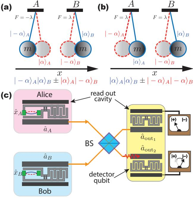
FIG. 1. (color online) (a) and (b) Schematic representation of different types of entangled cat states of two suspended masses moving harmonically along  $x$ -axis.  $\alpha$  is the displacement amplitude from the equilibrium position. (c) Sketch of a possible experimental implementation with quantum electromechanical circuit.
