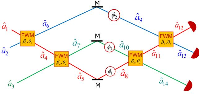
FIG. 2: (Color online) The schematic diagram of the  $SU(1,2)$  interferometer.  $\hat{a}_i$  ( $i = 0, 1, \dots, 14$ ) denote the different light beams in the interferometer.  $\beta_i$  and  $\theta_i$  ( $i = 1, 2, 3, 4$ ) describe the strength and phase shift in the different four-wave-mixers (FWMs) processes.  $\phi_i$  ( $i = 1, 2, 3$ ): phase shifts;  $M$ : mirrors.
