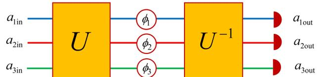
FIG. 1: (Color online) General three-port balanced interferometer.  $\phi_i$  ( $i = 1, 2, 3$ ): phase shifts.
