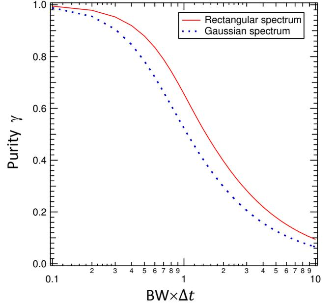
FIG. 1. (color online). Quantum-state purity  $\gamma$  as a function of  $BW \times \Delta t$ , the product of biphoton bandwidth (BW) and the trigger-photon detection response time ( $\Delta t$ ). The solid (red) curve is calculated from the rectangular-shape spectrum, and the dotted (blue) curve from the Gaussian-shape spectrum with BW as the full width at half maximum.
