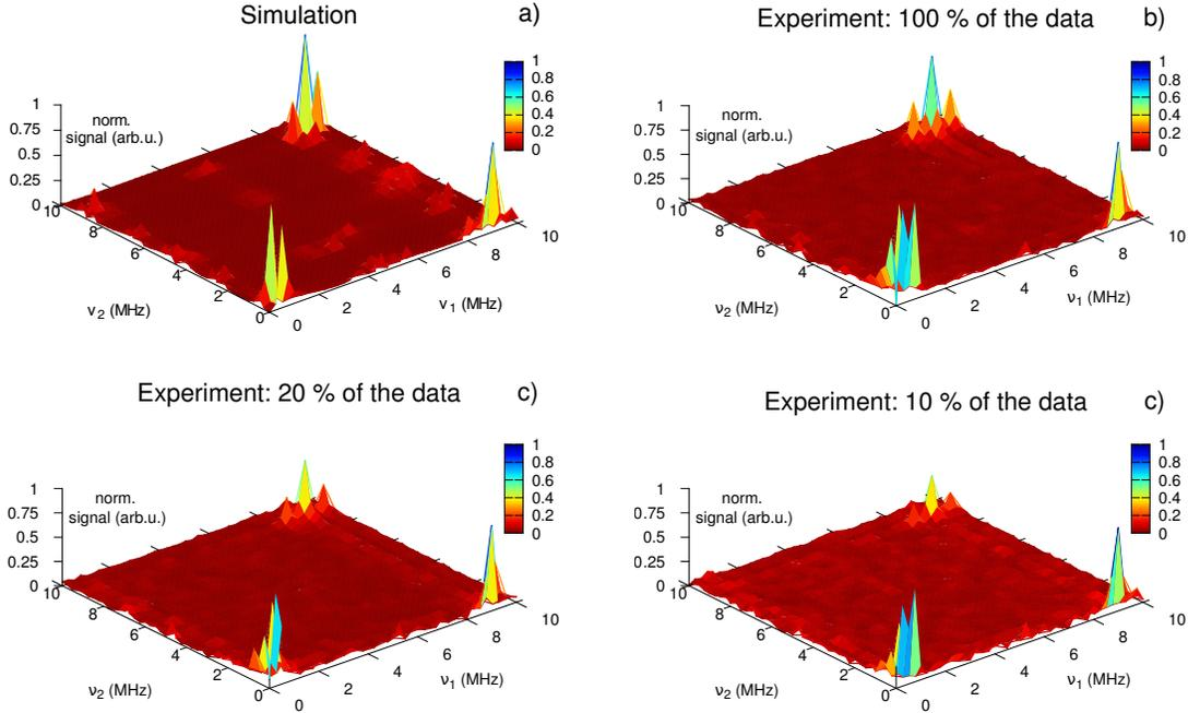
**Figure 3.** 2D ESEEM simulation and experimental data with a single NV coupled to a single  $^{13}\text{C}$  nuclear spin. (a) Simulation using the spin Hamiltonian (6) and (7). (b) Fourier transform of the complete set of the experimental data points. Fourier transform of 20% (c) and 10% (d) of the data in the time domain. Here we again can recover the spectral information by keeping small amount of the experimental data.
