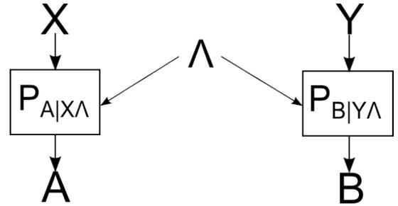
FIG. 1. Two boxes are programmed by a hidden common strategy  $\Lambda$ . The boxes are given inputs  $X$  and  $Y$  and return outputs  $A$  and  $B$ . There is the possibility for nondetection events, in which case the corresponding output variable takes the value  $\emptyset$ .
