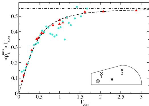
FIG. 3: Same as Fig. 2 for the cases of  $\mathcal{T}$  violation in the experiment (turquoise dots) and the GUE in the RMT simulations (red triangles). Inset: same as in Fig. 1. In addition a magnetized ferrite (black disk) was inserted to enforce  $\mathcal{T}$  violation.
