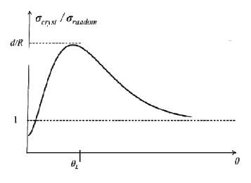
Fig.5. Orientation dependence of single-photon annihilation at the positron entrance angle  $\theta$ .
