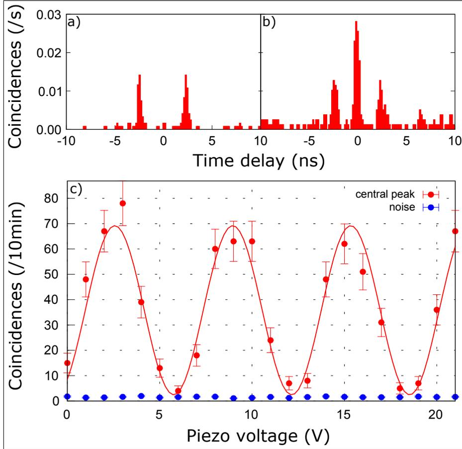
Figure 4: Results of the Franson experiment: a) and b) histograms of the coincidence rate for two different phase settings, chosen to minimize and maximize the central peak ; c) two photon interference: the coincidence count rate of the central peak is plotted as a function of the phase  $\phi$ . The internal estimated pump power is  $273 \mu\text{W}$ . The line show the fitting curve used to estimate the visibility  $V_{net} = 95.6 \pm 3.7\%$ .
