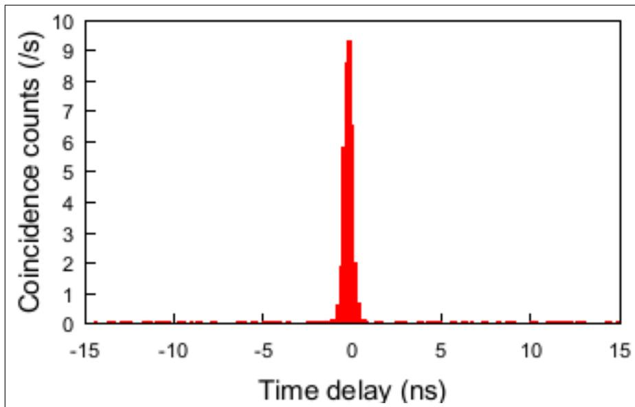
Figure 2: Coincidence histogram of TE/TM photons passing through the FBG filter centered at  $1.566 \mu\text{m}$  at  $T= 20.1^\circ\text{C}$ . The data were accumulated during 100 s with a sampling resolution of 164 ps.
