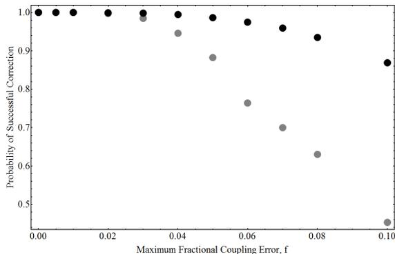
FIG. 3. In the minimal working example, we test faults due to coupling errors, altering each uniformly at random in the range  $J_n(1-f)$  to  $J_n(1+f)$ , assessing the probability of successful corrections and averaging over 1000 different instances (black) or the minimum success probability (grey).
