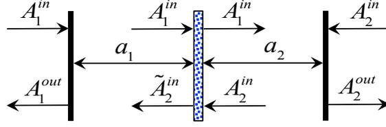
**Figure 2. Schematic diagram of the input and output modes of the system.** The two cavity modes  $a_1$  and  $a_2$  exert a strong dynamical influence on one another via phase locking by the oscillating mirror which effectively acts as a partly reflecting and partly transmitting mirror.
