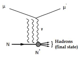
Figure 1. Deep inelastic muon-nucleon scattering
