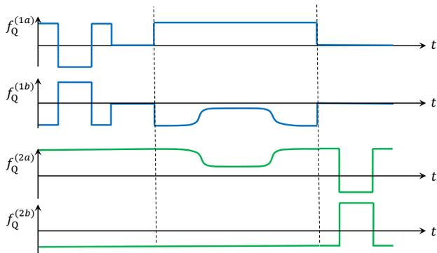
FIG. 5. **Pulse sequence for encoded CPHASE gate.** This schematically shows a sequence for CPHASE gate in Eq. (6). Single qubit phase gate is implemented with three step Euler rotations, and Pauli X and identity gates are implemented as a single rotation. The two vertical dashed lines separate single qubit gates and two-qubit adiabatic operation.
