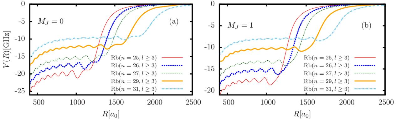
FIG. 2. For the Rb-KRb molecule, the energetically lowest-lying states with  $M_J = 0$  and  $M_J = 1$  evolving from the Rb( $n, l \geq 3$ ) Rydberg manifold, for  $n = 25, 26, 27, 29$ , and  $31$ , and KRb in the rotational ground state  $N = 0$  are shown. To facilitate the comparison, the zero energy has been set to the energy of the Rb( $n, l \geq 3$ ) degenerate manifold and the KRb( $N = 0$ ) level.
