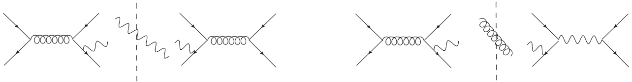
FIG. 4: Schematic representation of the two different kinds of insertion operators, representing QED singularities (l.h.s.) and QCD singularities (r.h.s.). This also illustrates the two different types of real emission contributions.
