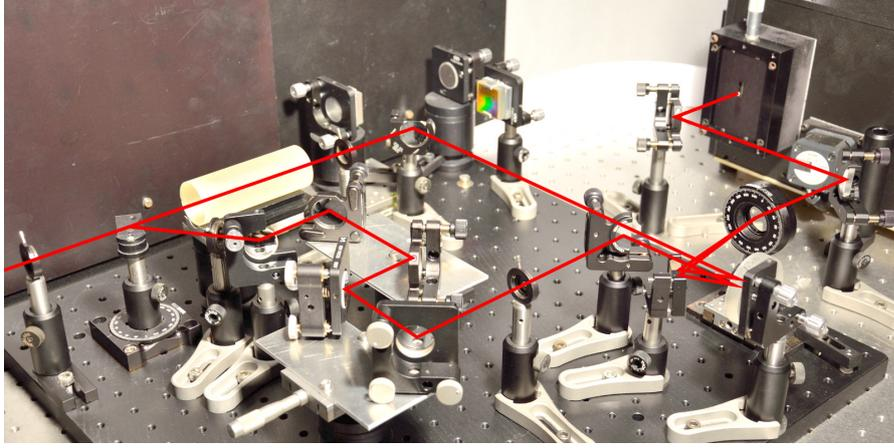
FIGURE 1. Measurement setup in self-diffraction spectral interferometry.
