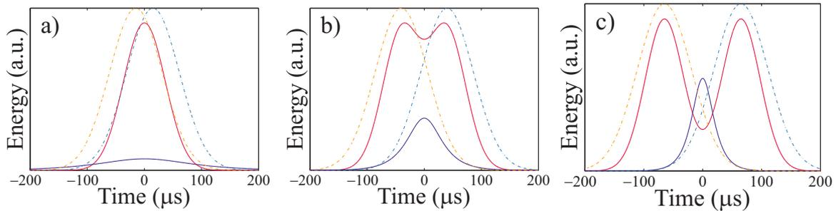
**Figure 2. Time dependence of the adiabatic criterion** The couplings (left side of (8), blue) and the energy splitting (right side of (8), red) are shown for a fixed pulse length of  $100 \mu\text{s}$  and (a) a delay time of  $30 \mu\text{s}$ , (b) a delay time of  $80 \mu\text{s}$  and (c) a delay time of  $130 \mu\text{s}$ . The dotted lines represent the pulses.
