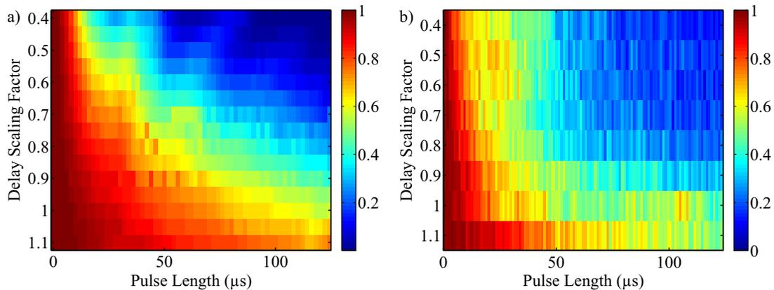
**Figure 5. Transfer efficiency for different delay scaling factors and pulse length for blue sideband transitions.** a) Simulation and b) experimental results of the STIRAP transfer, where red corresponds to no and blue to complete transfer. For the simulations and the measurements the ion was initialized in the ground state of motion and the pulse length was scanned for different delay scaling factors  $s$ .
