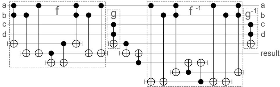
Fig. 7: The resulting reversible network for computing the function  $h(a,b,c,d) = f(a,b) \oplus g(c,d)$ . The sub-circuit labeled with “f” is obtained from the MDD shown in Figure 6. Similarly, a sub-circuit for  $g$  is obtained from an MDD for  $g$ , which is an AND function. The final result is copied out into the “result” wire and then cleanup is performed by running the circuits for  $f$  and  $g$  in reverse.
