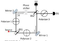
FIGURE 2. Quantum Eraser Setup
