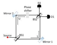
FIGURE 1. MZI setup with a phase shifter in the U path
