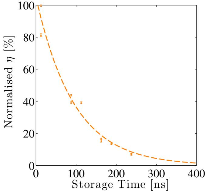
FIG. S2: We measured the memory lifetime by storing input pulses with average photon number  $\sim 10$  and recording the average number of retrieved photons, for a range of storage times. We extract a memory lift time of  $95 \pm 7$  ns from the exponential decay.
