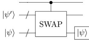
Here, the top qubit gets postselected onto  $|0\rangle$  with fidelity  $1 - O(1/\sqrt{2^n})$ , the middle register is discarded, and the bottom register is postselected onto  $|\psi\rangle$ , an operation we denote by  $\boxed{|\psi\rangle}$ .
