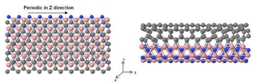
**Figure 3.** Left: A Super Cell of hetero-bilayer nanoribbons of boron nitride/graphene which contains 240 atoms. Right: A hetero-CNT obtained by relaxing the structure on the left.
