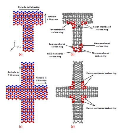
**Figure 2.** (a) A T-branched structure made by sculpting an AB-stacked bilayer. The structure is periodic in the horizontal direction. (b) The resulting T-branched CNT structure obtained by relaxing the bilayer ribbon of figure 2a. (c) A cross-like structure made by sculpting an AB-stacked bilayer. The structure is periodic in the horizontal and vertical direction. (d) A relaxed cross-like carbon nanotube structure obtained by relaxing the bilayer ribbon in figure 2c.
