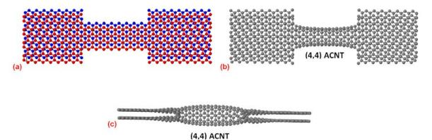
**Figure 4.** Fig 4a shows a finite AB-stacked BiGNR whose ends are connected to bilayer graphene electrodes; the unit cell contains 644 carbon atoms. Figs 4b and 4c show two views of the structure after relaxation, which comprised a CNT in the central region, attached to bilayer graphene 'electrodes'.
