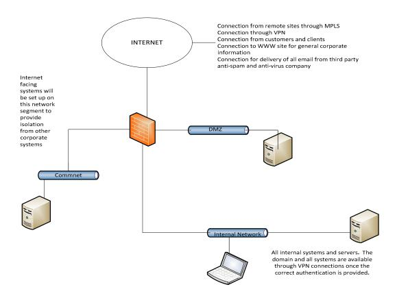
Figure 2: Basic Network Architecture
