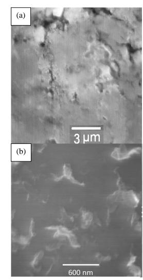
**Fig. 5** The SEM images of GRPPy sample before (a) and after (b) field emission test
