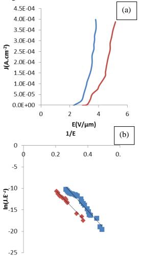
**Fig. 9** (a) Current density vs. applied field plot of composite samples on composite side (blue) and AAO membrane side (red), and (b) the Fowler-Nordheim plots developed based on the same data.
