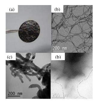
**Fig. 1** (a) The composite sample pressed into a disk for field emission measurements and (b) TEM images showing the raw carbon nanotubes, (c) formation of a layer of polypyrrole around nanotubes and (d) the graphene sheets embedded inside polypyrrole particles. The dotted line is used to show the boundary of the composite particle.
