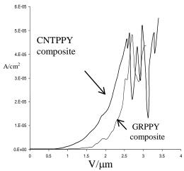
**Fig. 4** Current density vs. applied field graphs of CNTPPy and GRPPy.
