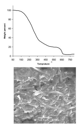
**Fig. 2** Thermogravimetric analysisof PPy/CNT (top) and SEM image (bottom) of a PEDOT/CNT composite.
