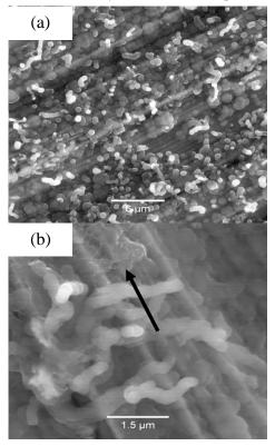
**Fig. 3** SEM images showing the surface of (a) the sample prepared by 10 CV cycles, and (b) the sample after 2 CV cycles, the arrow shows an area of carbon nanotubes with no polypyrrole coating.
