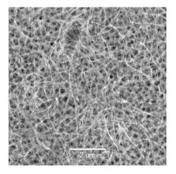
**Fig. 10** The SEM images of composite sample deposited on AAO membrane after field emission test
