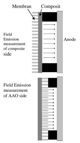
**Figure 8** The schematic view of the field emission measurement cells for testing both composite and AAO sides
