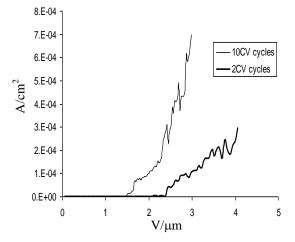
**Fig. 7** Current density vs. applied field plot of CNTPPy samples prepared by the electropolymerization process.
