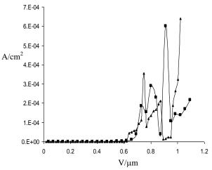
**Fig. 6** Current density vs. applied field graphs two of CNT/PEDOT samples with the same composition
