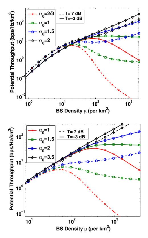
Figure 3: Potential throughput vs. BS density for 2D (top) and 3D (bottom) network topologies. Parameters are the same as for Fig. 2.
