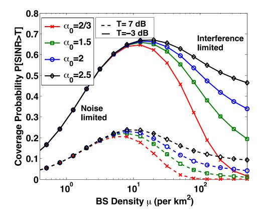
Figure 2: Probability of coverage vs. BS density (Poisson distributed, average per km<sup>2</sup>) in the 2D plane for SINR threshold T = 0.5 (-3dB) and 5 (7 dB), close-in path loss exponent  $\alpha_0$ , and with  $R_c$  = 100 m and  $\alpha_1$  = 4. The noise is set in each case such that the SNR=20 dB at  $R_c$ . There is Rayleigh fading, but no shadowing or sectoring.
