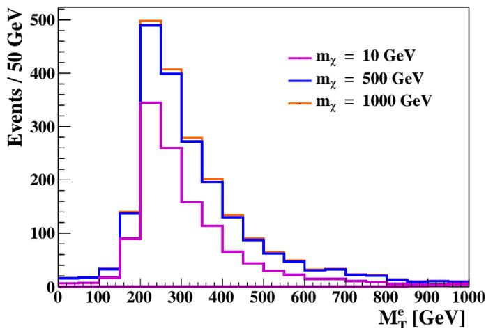
**Figure 3.**  $M_T$  distribution for  $m_{\eta_u} = m_{\eta_d} = 200$  GeV,  $g = 1$ ,  $m_\chi = 10, 500, 1000$  GeV in the  $t$ -channel model, at 14 TeV and  $\mathcal{L}_{int} = 3000 fb^{-1}$ . It can be seen that the distribution is independent of DM mass.
