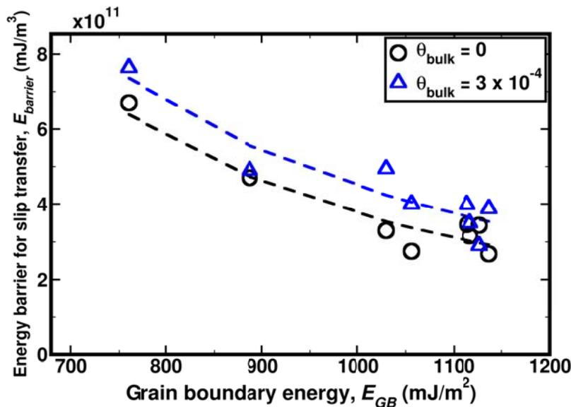
**Figure 6:** The effect of hydrogen on the slip transmission barrier through the <111> STGBs.
