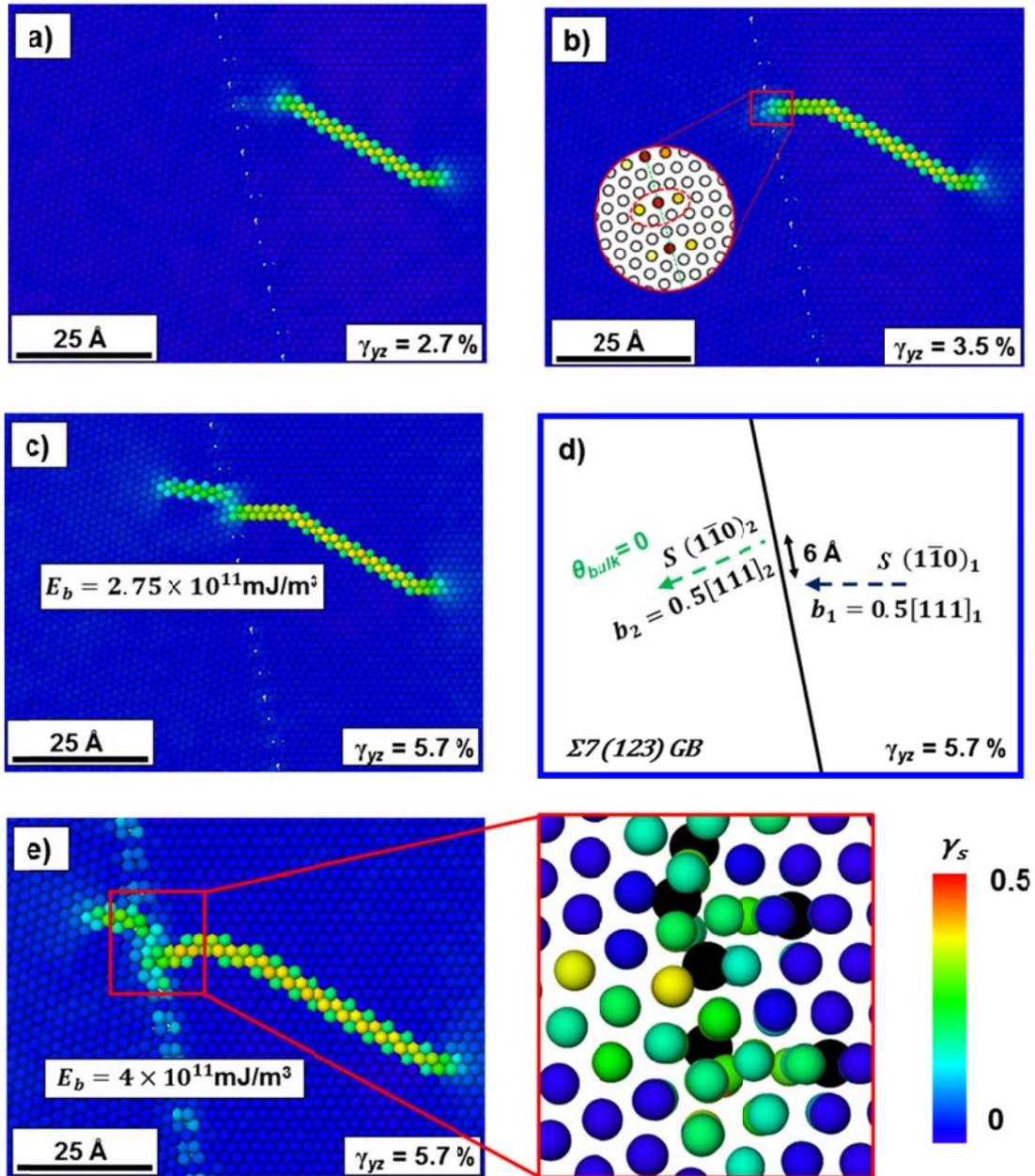
**Figure 3:** a-d) The interaction of a screw dislocation with the  $\Sigma 7$  (123) GB under the applied shear strain ( $\gamma_{yz}$ ) along the Burgers vector direction. The inset b) shows the magnified GB structure colored according to the atomic volume estimated by the Voronoi tessellation as
