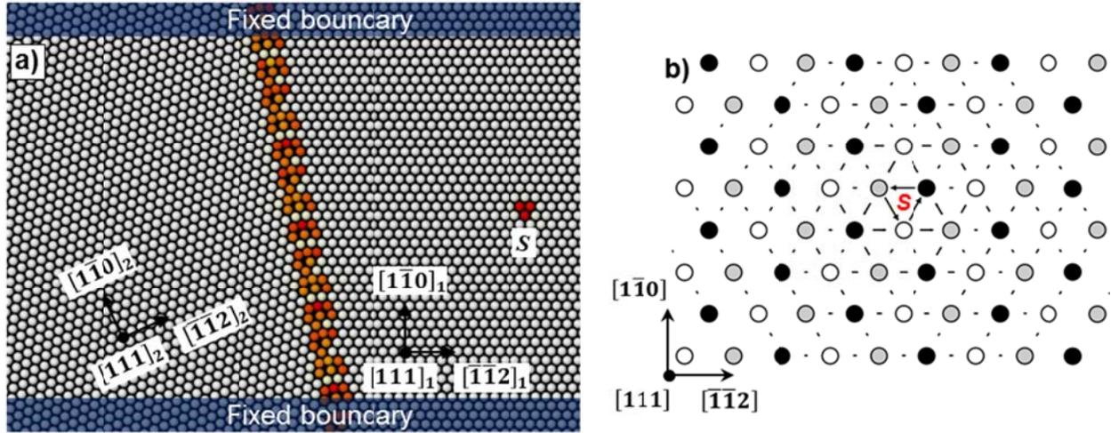
**Figure 2:** a) A schematic representation of the atomistic model employed to study the interaction between a screw dislocation (core marked as “S”) and the  $\langle 111 \rangle$  STGB in  $\alpha$ -Fe. b) Differential displacement map of the compact core in Fe and the atomic colors emphasize different (111) planes.
