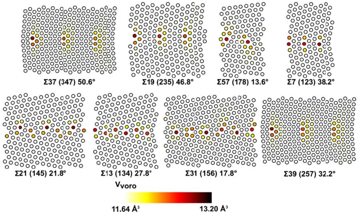
**Figure 1:** The  $\langle 111 \rangle$  symmetric tilt GB structures in  $\alpha$ -Fe used in this work. Atoms are colored based on the atomic volume estimated by Voronoi tessellation on a scale of  $11.64 \text{ \AA}^3$  to  $13.20 \text{ \AA}^3$ .
