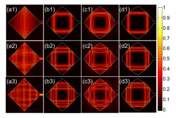
FIG. 3 Calculated magnetic field component  $|H_z|$  for the 0th-order, 1st-order, and 2nd-order symmetric transverse modes are presented in (a1)-(a3) at  $\delta = 0$ , (b1)-(b3)  $\delta = 0.5 \mu m$ , (c1)-(c3)  $\delta = 0.9 \mu m$ , and (d1)-(d3)  $\delta = 1.3 \mu m$ , respectively.
