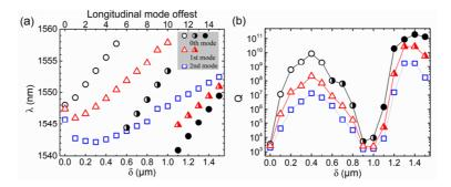
FIG. 2 (a) Resonance wavelengths around 1550 nm and (b) corresponding Q factors versus the deformation amplitude  $\delta$ . The variation of the longitudinal mode number is also traced in (a) for the square marked modes, and the open, half-filled, and solid symbols belong to different longitudinal modes at a certain  $\delta$ . The fundamental (0th-order), first-order (1st-order), and second-order (2nd-order) transverse modes are marked by circle, triangle, and square symbols, respectively.
