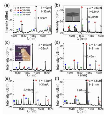
FIG. 4 (a)-(f) Lasing spectra for the CSR lasers with  $\delta$  of 0, 0.5, 0.9, 1.1, 1.3, and 1.5 µm, respectively. The 0th-order, 1st-order, and 2nd-order, and third-order (3rd-order) transverse modes are marked by circle, triangle, square, and pentagram symbols, respectively, with the open, half-filled, and solid symbols belonged to different longitudinal modes. Insets in (b) and (c) are a side-view SEM image after ICP etching and a top-view microscope image of a microlaser.
