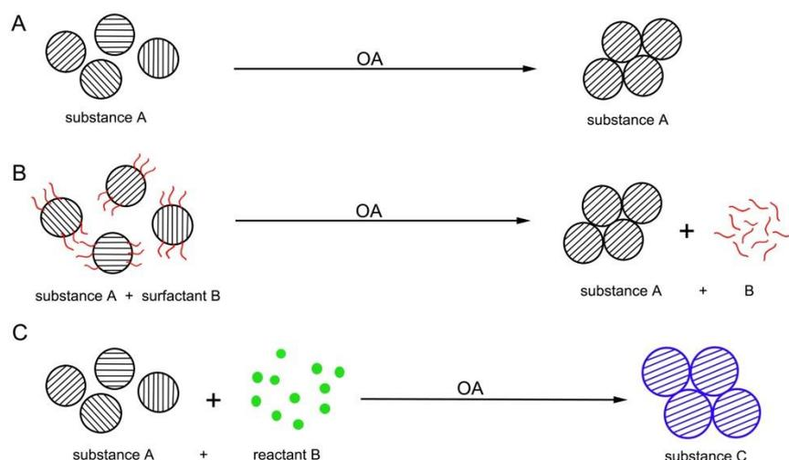
**Figure 1. Schematics of conventional OA processes (A and B) and chemical reaction directed OA process (C).** (A) The oriented alignments of primary nanoparticles and fusion to form a single crystal. (B) With the assistance of surfactants (red wavy lines) a single crystal grows via oriented
