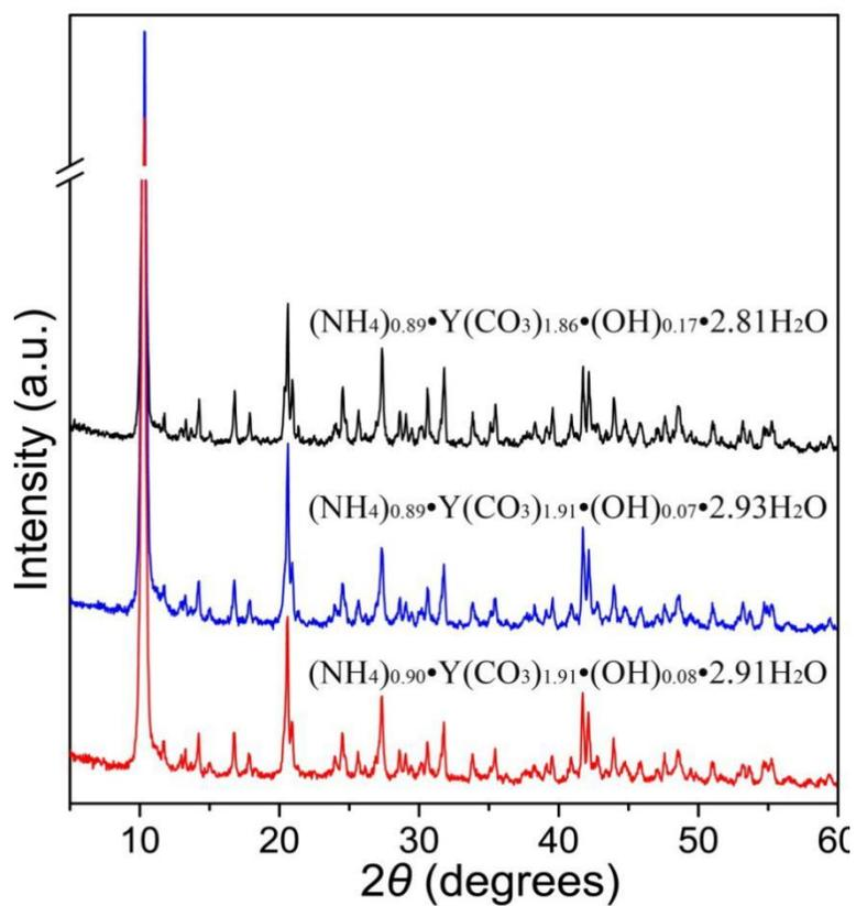
**Figure S18.** Powder XRD patterns of Y2 micron-sized sheets with slight differences in chemical compositions synthesized under different molar ratio of total  $\text{NH}_4\text{HCO}_3$  to  $\text{Y}(\text{NO}_3)_3$  (see **Table S1**). No obvious differences in the patterns are observed, which indicate that there is no apparent change in its crystal structure.
