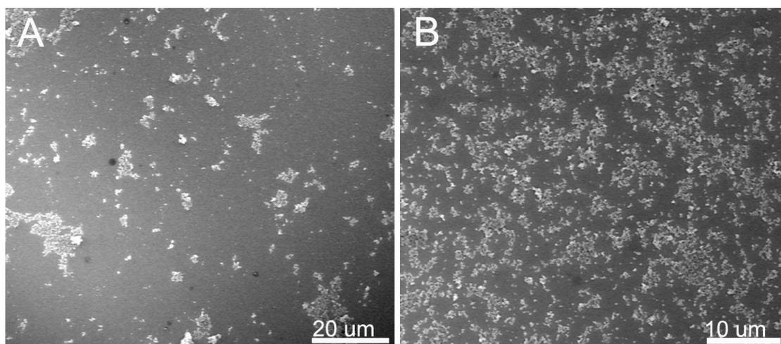
**Figure S10.** FESEM images of the samples synthesized by introducing (A) NaOH and (B)  $\text{NH}_4\text{OH}$  aqueous solutions into  $\text{Y}_2(\text{CO}_3)_3 \cdot 2\text{H}_2\text{O}$  nanoparticle suspensions. No micron-sized or nano-sized sheets were obtained, indicating the key role of the double-salt reaction in the OA process.
