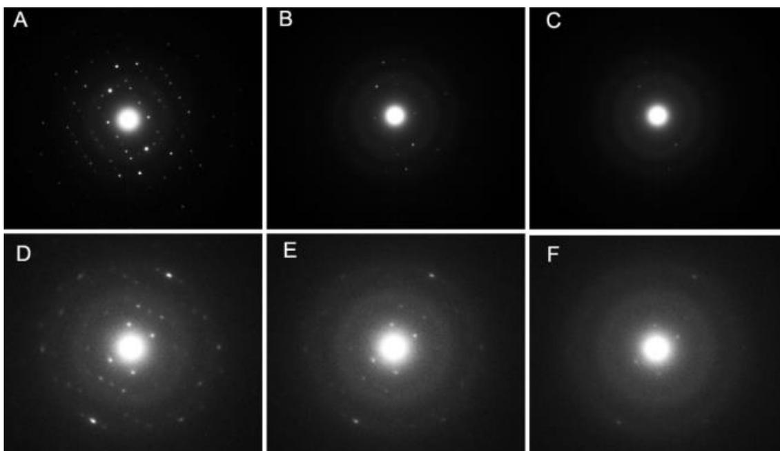
**Figure S3.** Evolution of SAED patterns of (A-C)  $\text{NaY}(\text{CO}_3)_2 \cdot 6\text{H}_2\text{O}$  sheet within ~ 30 seconds and (D-F)  $(\text{NH}_4)_2\text{Y}(\text{CO}_3)_2 \cdot \text{H}_2\text{O}$  sheet within ~ 10 seconds due to the beam damage. Such rapid decomposition of  $(\text{NH}_4)_2\text{Y}(\text{CO}_3)_2 \cdot \text{H}_2\text{O}$  sheet leads to difficulty to obtain the lattice-fringe image.
