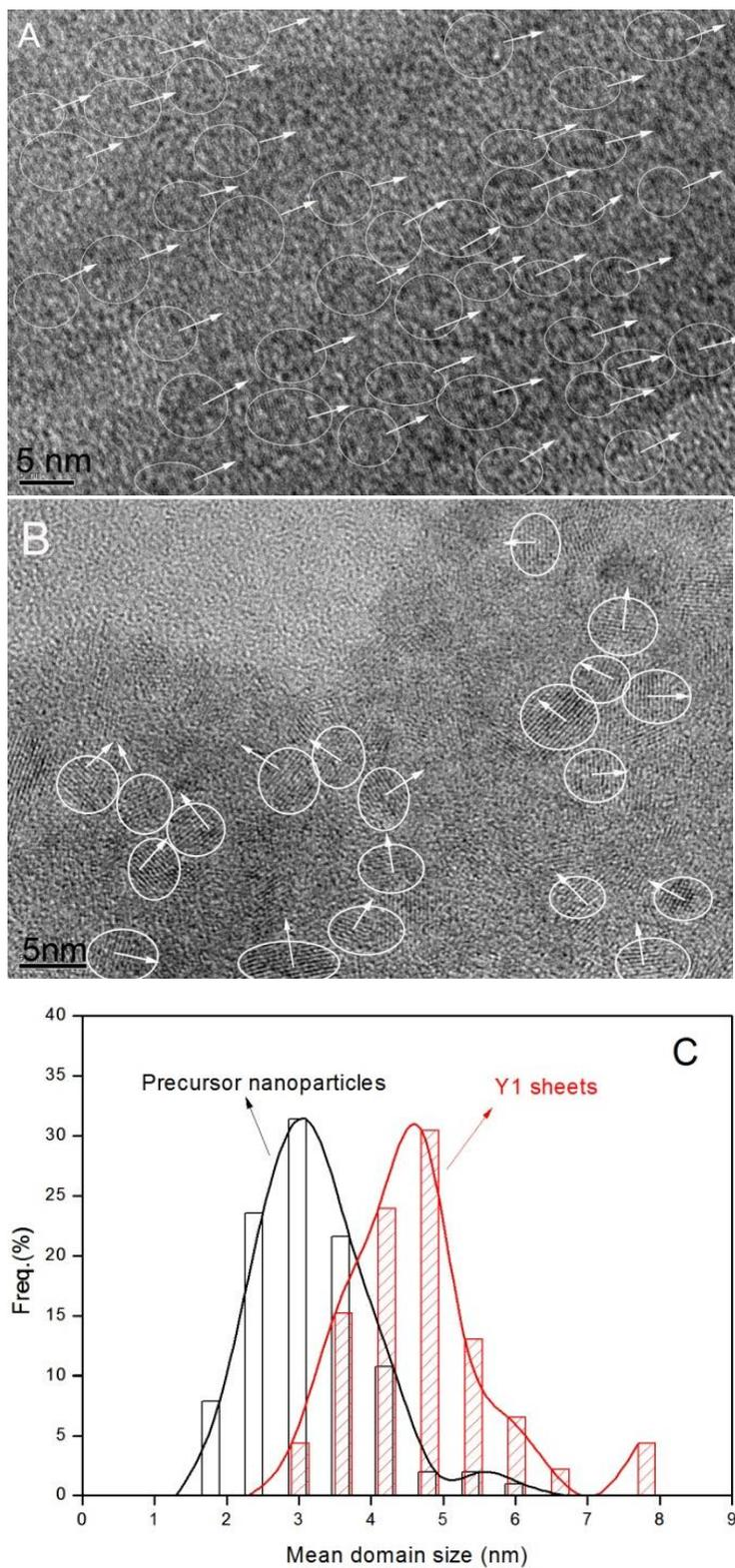
**Figure S2.** High resolution TEM images of the NaY(CO<sub>3</sub>)<sub>2</sub>·6H<sub>2</sub>O sheets (A) and precursor Y<sub>2</sub>(CO<sub>3</sub>)<sub>3</sub>·2H<sub>2</sub>O particles (B); The domain size distributions of the precursor nanoparticles and Y1 sheets (C).
