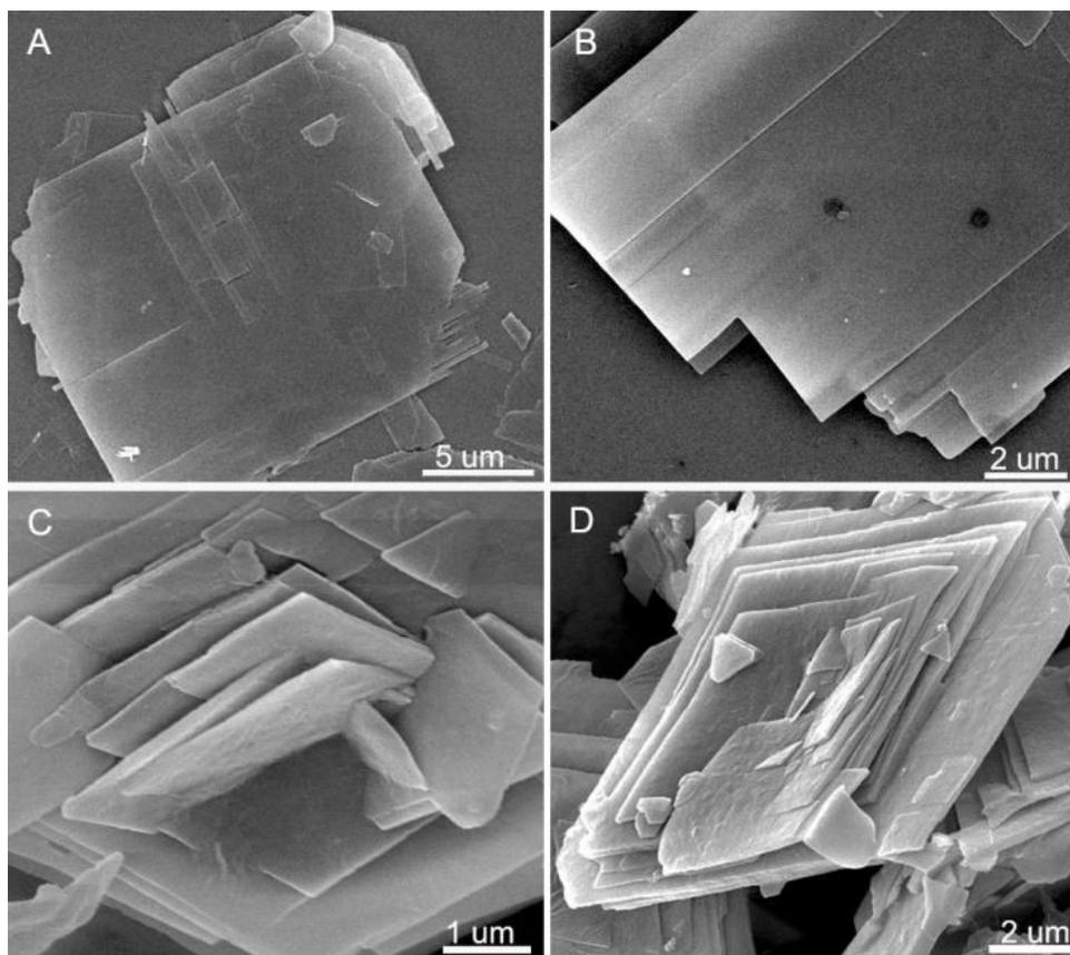
**Figure S1.** FESEM images of the obtained sheets. (A-B)  $\text{NaY}(\text{CO}_3)_2 \cdot 6\text{H}_2\text{O}$ , (C-D)  $(\text{NH}_4)\text{Y}(\text{CO}_3)_2 \cdot \text{H}_2\text{O}$ .
