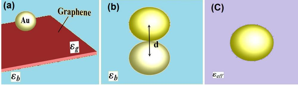
Fig. 2. (a) Particle on graphene layer, where  $\varepsilon_g$  and  $\varepsilon_b$  are the dielectric permittivity of graphene and surrounding medium. (b) Induced charge on the graphene can be imagined as surface charge on a pseudoparticle that interacts with the particle. (c) The model: nanoparticle in a homogeneous medium with permittivity  $\varepsilon_{eff}$ .
