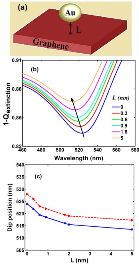
Fig. 4 : (a) Nanoparticle above a graphene layer. (b) Dependence of resonance on gold nanoparticle-graphene separation. The arrow shows the movement of dip position as the gap between nanoparticle and graphene becomes wider. (c) Calculated shifts of dip position using the effective permittivity (solid line) and FDTD simulation (dashed line).
