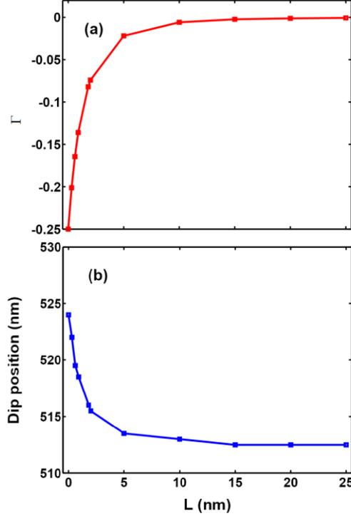
Fig. 5. (a) Dependence of  $\Gamma^k$  and dip position on gold nanoparticle-graphene separation.
