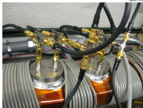
Figure 33. Photo of Shielded Pickups installed at 15E with the installed solenoid winding
